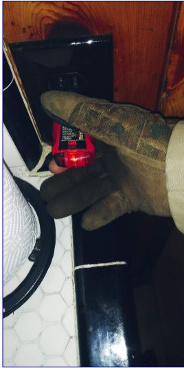
Several interior three prong outlets have not been grounded correctly
